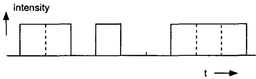
Fig. 10.1. Non-return-to-zero format: a 110100111 sequence
